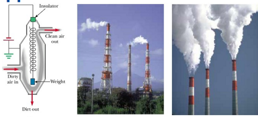
Figure 25.28 (a) Schematic diagram of an electrostatic precipitator. The high negative electric potential maintained on the central coiled wire creates an electrical discharge in the vicinity of the wire. Compare the air pollution when the electrostatic precipitator is (b) operating and (c) turned off.
